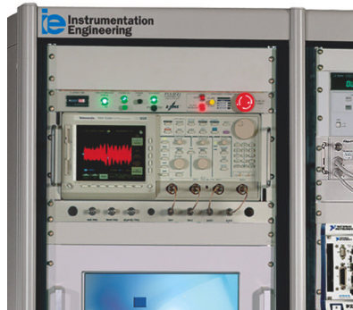
The traditional short and deep oscilloscope form factor saves rack space over tall scopes designed for the bench. Courtesy of Instrumentation Engineering.
